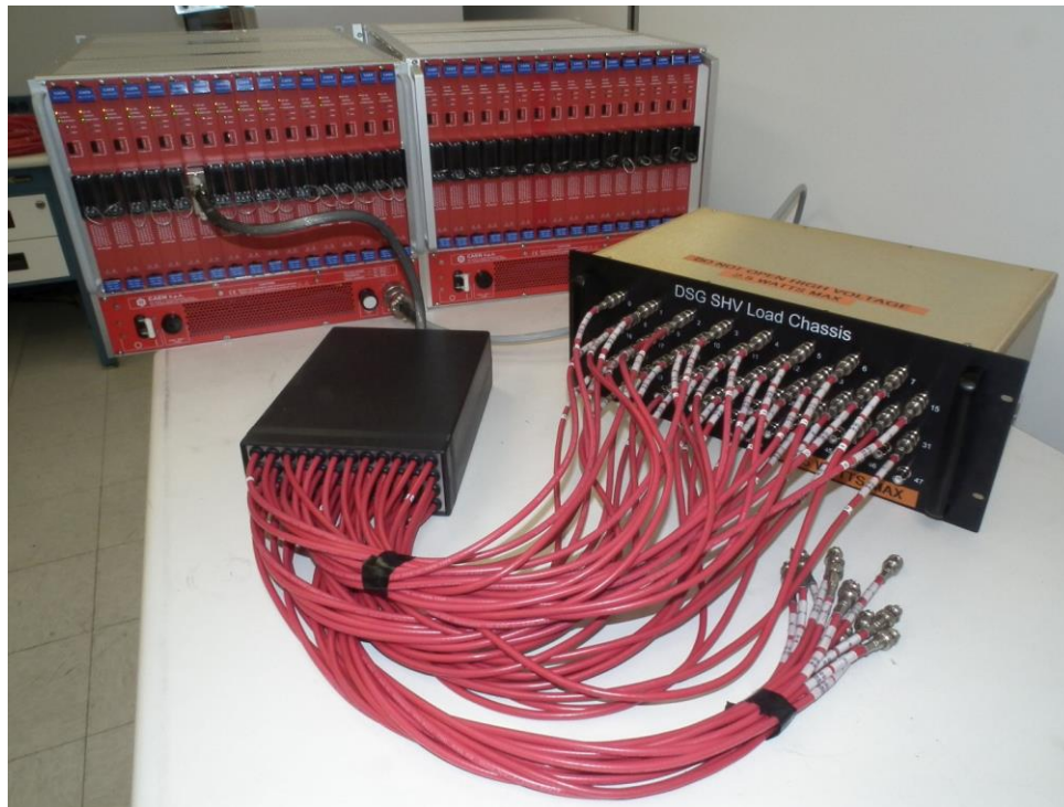
CAEN HV test set up with two fully populated crates and one card connected to a Radiall-to-SHV adapter chassis and then to the Load Chassis.
